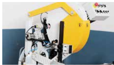
01 Heavy Duty HSS Blade with Automatic liquid cooling system
