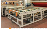
10 Multidirectional cross conveyor sends the mattress to the rolling unit or send it to other direction for only-wrapped mattresses
