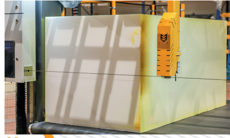
02 Servo controlled, automatic center knife support for high quality and high-speed cutting operation
