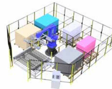
RobET-SFP Automatic Feeding and Assembly Robot
