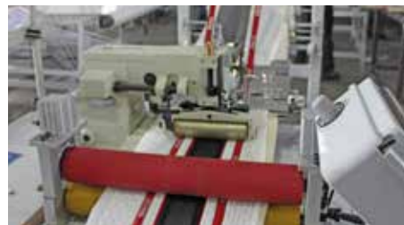
01 Servo driven puller cylinders
