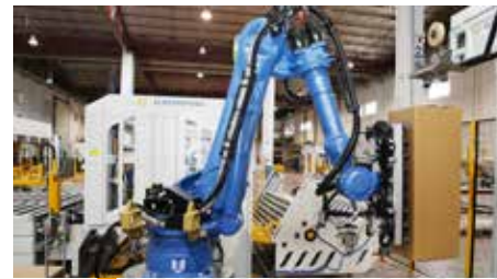
02 Auto box sorting and stacking to multiple pallets or conveyor exit
