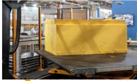
01 Automatic turntable for 3D parts.
