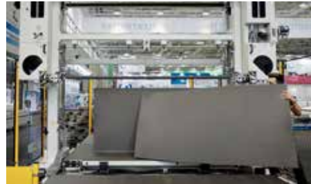
02 Able to clean sides, top and bottom of the foam block
