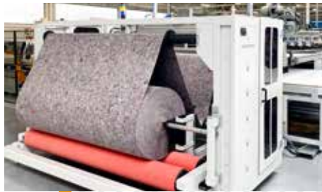
11 Optional Felt Cutting and Assembling System (FEL-X2)
