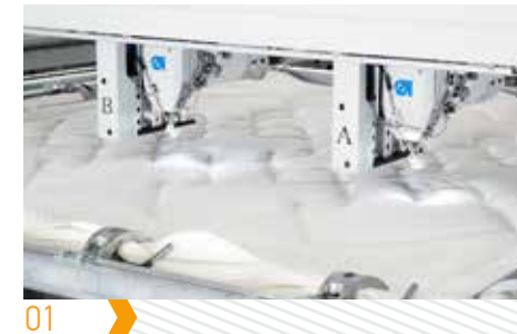
01 Heavy Duty Durkopp Adler 867 Sewing Heads with 32mm XXL Bobbin
