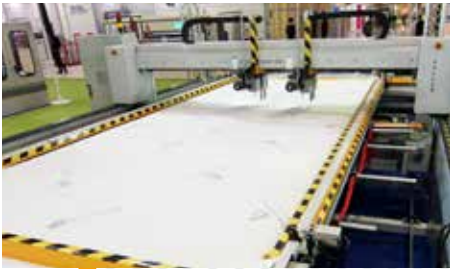
08 Adjustable material tension from both sides Enden ve boydan ayarlanabilen malzeme gerdirme sistemi
