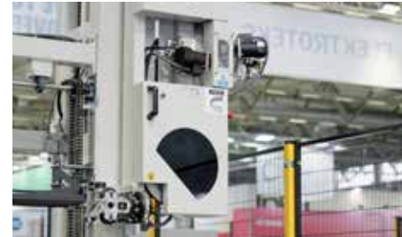
03 Automatic Blade Grinding: Programmable blade grinding operation
