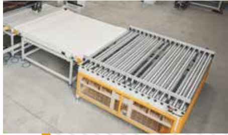
02 Self-aligning infeed conveyor
