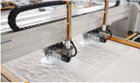
02 Automatic top and bottom thread cutting within 0.5 Seconds Otomatik alt ve üst ip kesme sistemi
