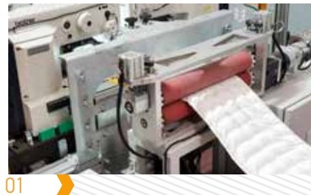
01 Reliable BROTHER KE-430 tacking heads
