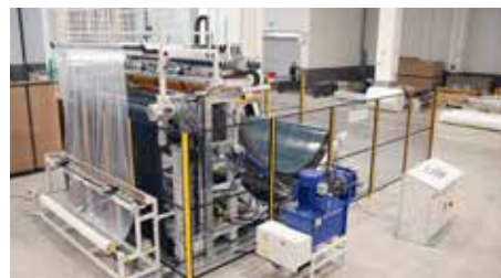
02 Double-sided synchronized mechanical conveyor tightening mechanism
