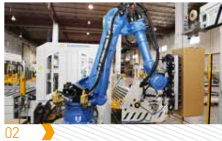
02 Auto box sorting and stacking to multiple pallets or conveyor exit
