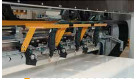
01 Oscillating center glue heads
