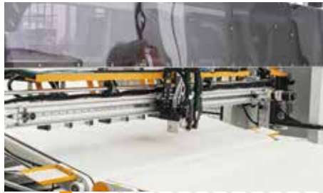
06 Self detection of mattress sizes: width, length, height
