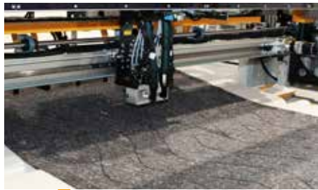
10 Equipped with laser sensors: no sensitivity for colors
