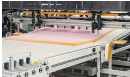
09 Servo motor driven conveyors and glue guns
