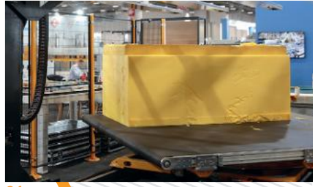
01 Automatic turntable for 3D parts.
