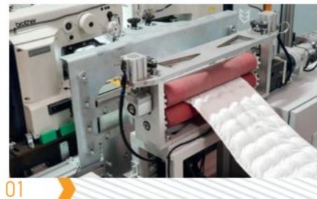
01 Reliable BROTHER KE-430 tacking heads
