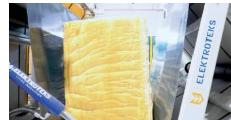
03 Able to compress and roll block foam as well.
