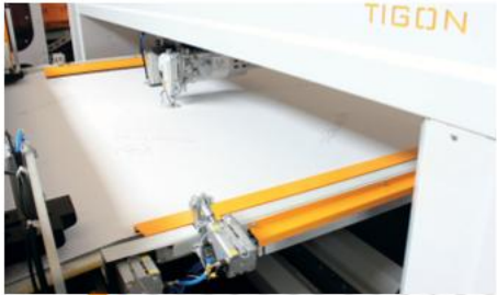
09 Adjustable material tension from both sides Enden ve boydan ayarlanabilen malzeme gerdirme sistemi
